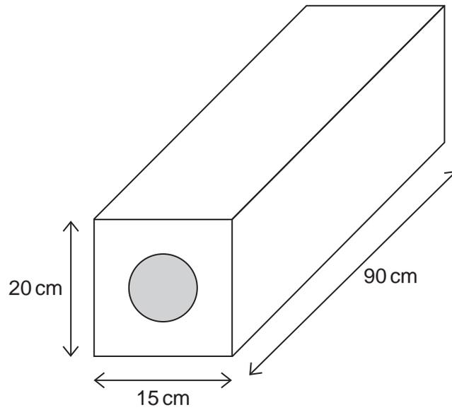
The block contains one steel cylindrical rod of length 90 cm.
